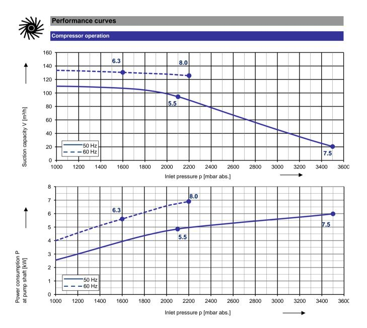
The characteristic curves are based on the evacuation of 100 % saturated air and an intake temperature of 20 °C. At a suction pressure of 1013 mbar abs. and a temperature of the operating liquid of 15 °C (water as operating liquid) the characteristic curv
