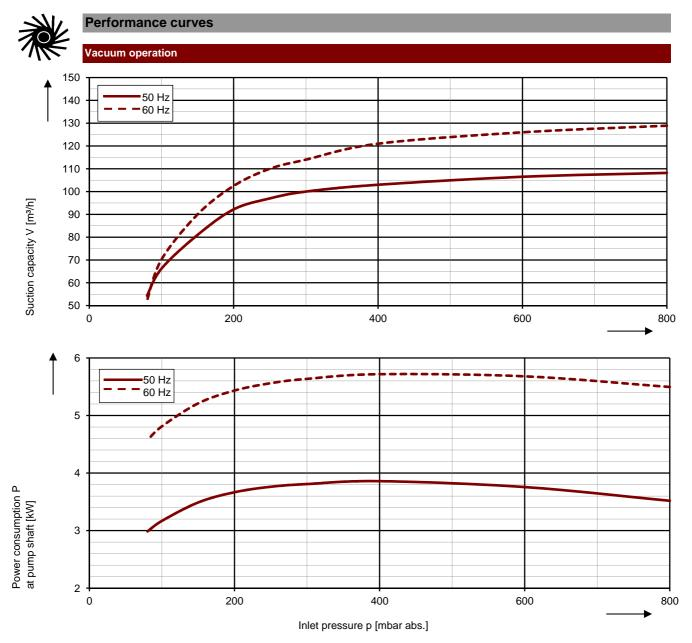
The characteristic curves are based on the evacuation of dry air and an intake temperature of 20 °C. At a suction pressure of 1013 mbar abs. (w ater as operating liquid) the characteristic curves will be achieved. The tolerance is  $\pm$  10 %.
