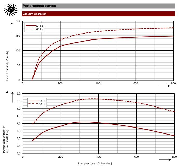
The characteristic curves are based on the evacuation of dry air and an intake temperature of 20  $^{\circ}$ C. At a suction pressure of 1013 mbar abs. (water as operating liquid) the characteristic curves will be achieved. The tolerance is  $\pm$  10 %.
