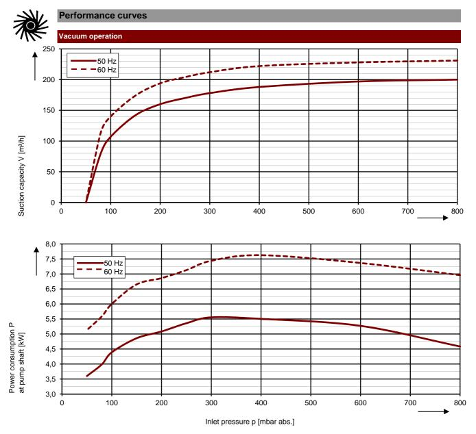
The characteristic curves are based on the evacuation of dry air and an intake temperature of 20 °C. At a suction pressure of 1013 mbar abs. (water as operating liquid) the characteristic curves will be achieved. The tolerance is  $\pm$  10 %.
