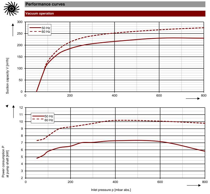
The characteristic curves are based on the evacuation of dry air and an intake temperature of 20  $^{\circ}$ C. At a suction pressure of 1013 mbar abs. (water as operating liquid) the characteristic curves will be achieved. The tolerance is  $\pm$  10 %.
