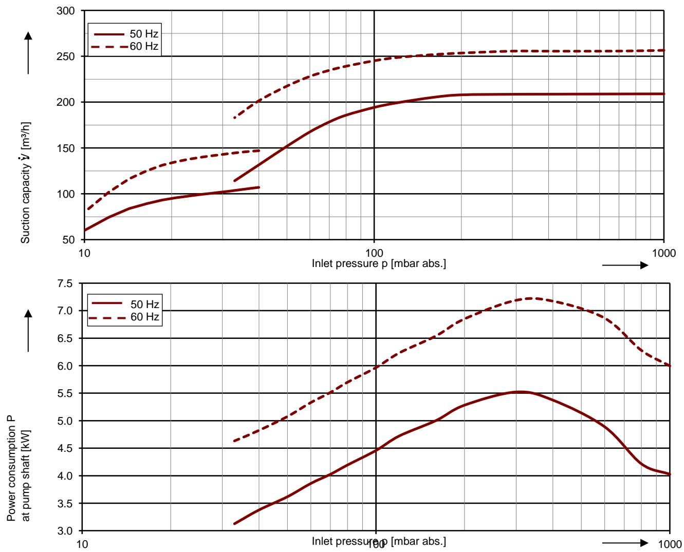
The characteristic curves are based on the evacuation of 100 % saturated air and an intake temperature of 20 °C. At a suction pressure of 1013 mbar abs. and a temperature of the operating liquid of 15 °C (water as operating liquid) the characteristic curves will be achieved. The tolerance is  $\pm 10\%$ .
