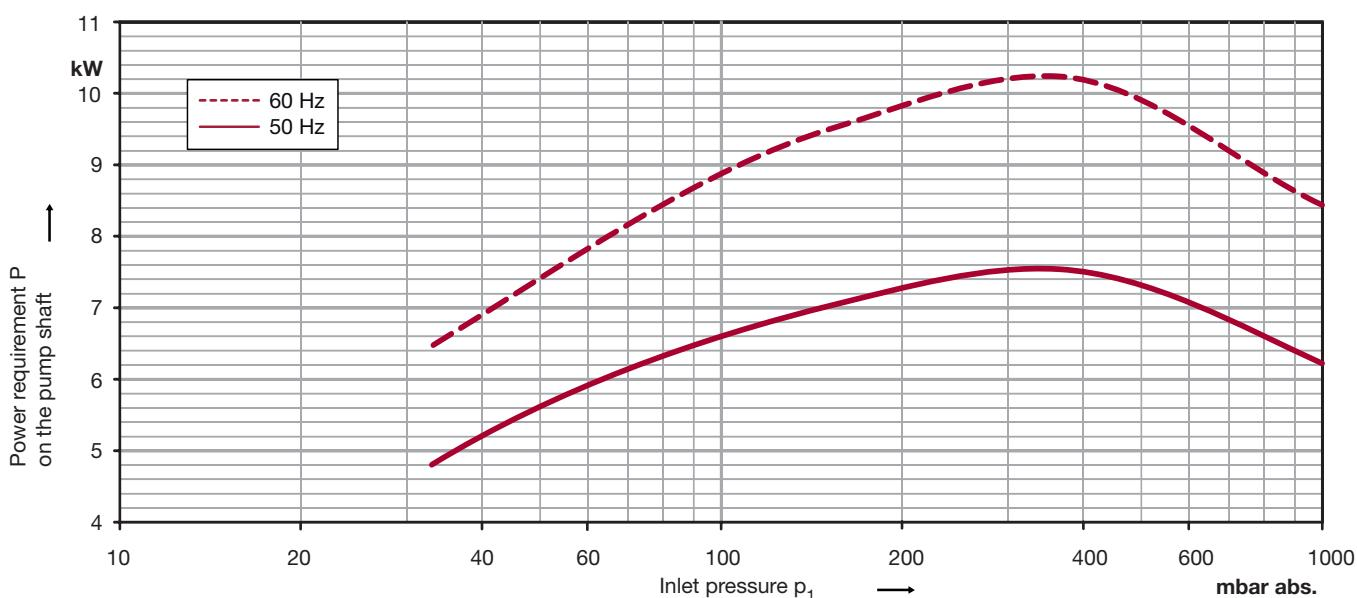
Vacuum pumps of the L-BV5 range are suitable for evacuating gases and wet vapours down to inlet pressures of 33 mbar abs. (97% vacuum). All these vacuum pumps are equipped with built-in cavitation protection. For operation below 80 mbar abs. the cavitation protection should be connected to protect the vacuum pump. All pumps L-BV5 are especially space-saving in their monoblock design. They are available in cast iron (standard color RAL 9006). The motor is painted as standard in RAL 9006.
