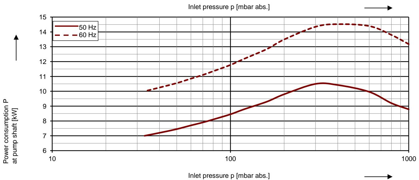
The characteristic curves are based on the evacuation of 100 % saturated air and an intake temperature of 20 °C. At a suction pressure of 1013 mbar abs. and a temperature of the operating liquid of 15 °C (water as operating liquid) the characteristic curves will be achieved. The tolerance is  $\pm 10\%$ .
